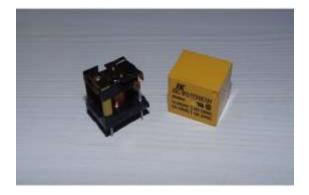
A Relay is a simple electromechanical switch. While we use normal switches to close or open a circuit manually, a Relay is also a switch that connects or disconnects two circuits. But instead of a manual operation, a relay uses an electrical signal to control an electromagnet, which in turn connects and disconnects another circuit.
