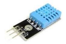
DHT11 humidity and temperature sensor is available as a sensor and as a module. The difference between this sensor and module is the pull-up resistor and power-on LED. DHT11 is a relative humidity sensor. To measurethesurrounding air this sensor uses a thermistor and a capacitive humidity sensor.
